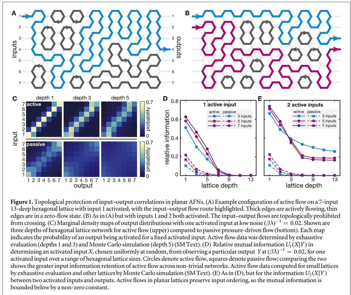
order of the inputs: if input 1 is activated and connects to output 3, say, then input 2 can only connect to output 4 onwards (figure 1(B)), in stark contrast to the linearity of passive network flow. This suggests that active flows may be particularly adept at retaining input configuration memory when more than one input is activated.
